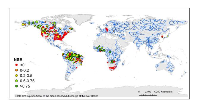
Figure 1. Nash-Sutcliffe efficiency of the validation globally (n= 335 stations). Circle size is proportional to the mean observed discharge at the river station.
