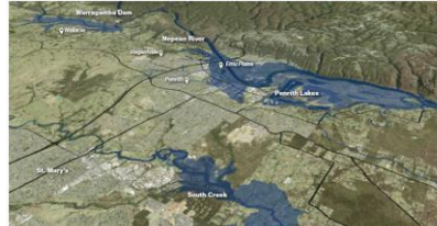
Image 1 Impact of a 1 in 500 chance per year flood at Penrith (similar in size to the largest flood on record – the 1867 flood).
